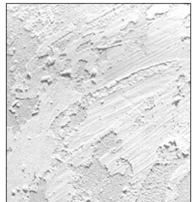
Flaking glass separator can cause the glass to crack. This is because the glass sticks to the shelf.
